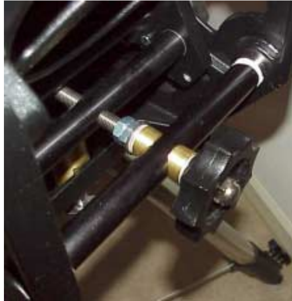
Altitude adjuster. The steel thrust bearings appear white in the photo. At the top right, teflon tape wrapped on the fixed bar prior to insertion in the shimmed hole is visible. At the top center, a slight ring of shim stock can be seen where the moving bar penetrates the tilt plate.
