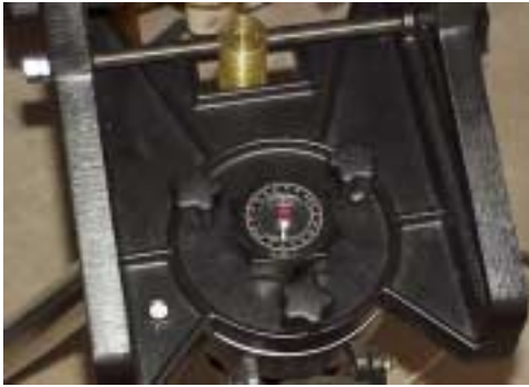
Knobs for attachment to tripod. Edge of teflon Disk is also visible. Note that I omitted one of the azimuth adjuster knobs.
